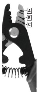
The SSF<sup>™</sup> Tri-Hole Fiber Optic Stripping Tool has three openings:
