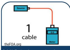
5. Cable Testing, place appropriate adapter onto OPM receiver, select and plug in cable (Single Mode or Multimode according to cable the cable being tested), between OLS and OPM.
