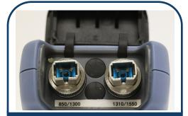
4. Plug REFERENCE cable into the appropriately labeled port on the OLS.
