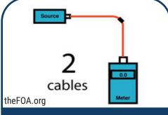
6. Cable Testing, place appropriate adapter onto OPM receiver, select and plug in two cables, one into OLS and other into OPM (Single Mode or Multimode according to the cable being tested). Link cables together with appropriate type adapter.
