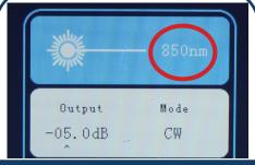
A. Wavelength on the OLS is displayed in the upper right corner of the screen. Set to desired value (press wavelength kev.)
