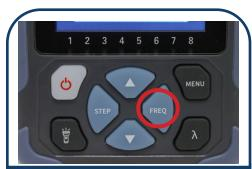
On the OLS press FREQ button until CW displays on the center of the screen below the wavelength (see step 1A image).
