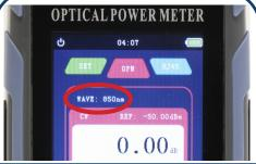
B. The OPM should be set to same wavelength as the OLS unit. Press the wavelength button until desired value appears.
