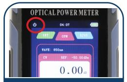
3. On both units ensure that the auto-power off funtion is not ON before setting any reference. If set to ON quick press the power button 1x to turn off the auto feature.
