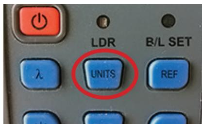
3. On the OPM, press the “UNITS” button until upper right portion of screen is blank and dBm is listed to the right of the main screen read-out (see step 1B image).
