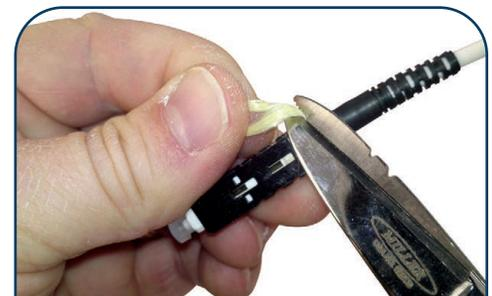
8. Hold Kevlar® and slide boot forward, keeping fiber straight. Thread boot onto rear one turn, cut Kevlar® closely to boot. Tighten boot until secure.
