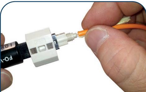
6. Insert cleaved fiber into the rear of connector until a "bow" is created and the light emitting from activator window is extinguished. Maintain forward pressure.
