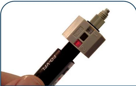
3. Place connector onto VFL. Press down firmly on top of activator housing to ensure the connector is in the "open" position. <sup>2</sup>
