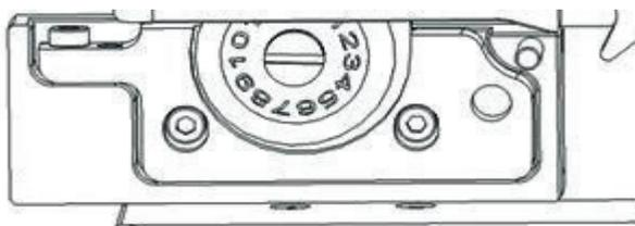
3. Carefully remove the blade carriage. Unscrew the blade fastening screw to remove the blade and insert new blade. Rotate blade and place number 1 on the uppermost position, then tighten the screws.
