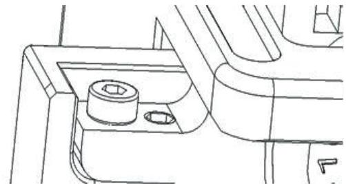
2. Loosen the blade clamping screw.
