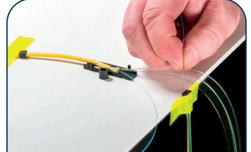
8. Insert each fiber through the matching colored furcation tube in the block until the fiber exits the far end of the tubing towards the floor.
