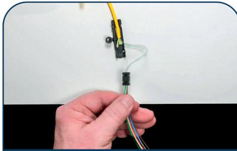
10. Remove furcation assembly from work surface. Holding all fibers on far end, slide assembly towards the jacket, leaving 1/2" or 12 mm between the block and the jacket.
