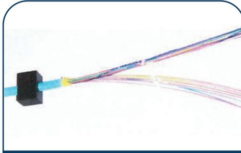
7A. For 24 strand fan out kit, separate fibers into 2 x 12 fiber color-coded bundles. Following directions in step 8 - 9, feed 12 fibers through each furcation assembly.
