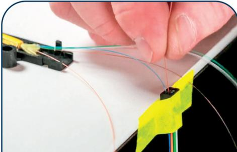
9. Ensure the fibers are not twisted around each other as they enter the block as this may cause attenuation from micro-bends at the point where they enter the block.
