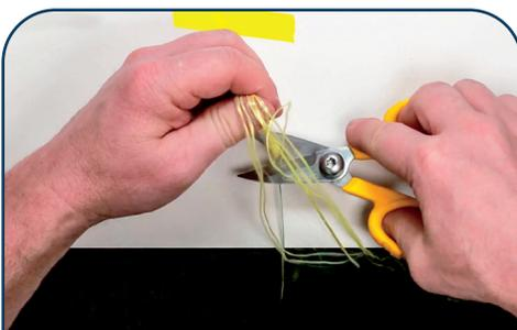
5. With fibers draping over the edge of the work surface, separate aramid yarns from fiber and cut yarns closely to the end of the cable jacket.
