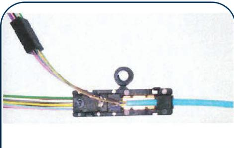
11A. For 24 strand fan out kit, insert second furcation assembly block into housing top.
