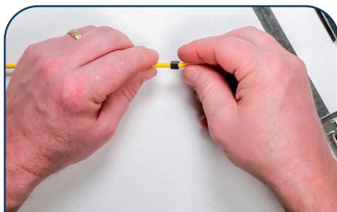
1. Slide the included properly sized holding clip for the cable being installed onto the cable jacket.
