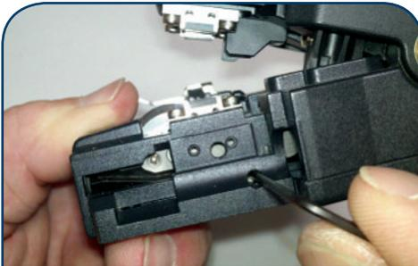
5. Locate the two "Blade Lock Screws". Using the Allen wrench loosen both screws, do not remove; screws need only be turned until they are loose.
