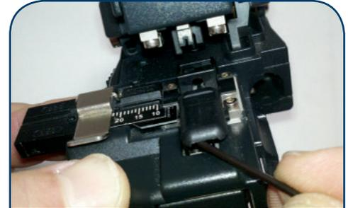
3. Using a small screwdriver or the Allen wrench, pry the blade cover up from the front slot as shown.
