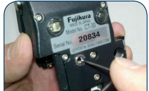
6. Locate the height adjuster screw on the bottom of the cleaver. Turn clockwise ¼ turn - raising the blade height. Tighten the two "Blade Lock Screws".
