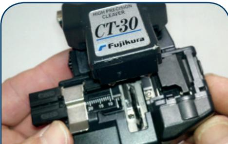
8. Install mm measurement sticker over existing sticker on cleaver - allowing cleave measurements up to 29mm.
