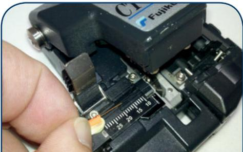
7. Attempt to cleave SSF™ fiber. If the cleaver does not successfully cleave the fiber repeat step #5 & #6. Repeat until the fiber is successfully cleaved.
