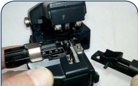
4. Remove blade cover and set aside. This piece will not be re-installed so place in cleaver case.
