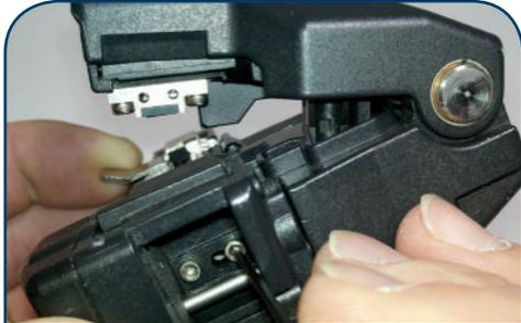
1. Using the cleavers Allen wrench included with cleaver, on the right side of cleaver remove the small fiber scrap box. Remove the two Allen screws.
