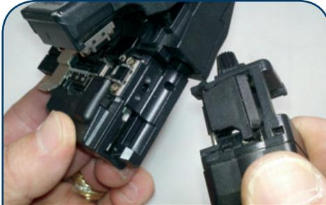
2. Once the screws are removed, remove the Fiber Scrap Collector and set aside.
